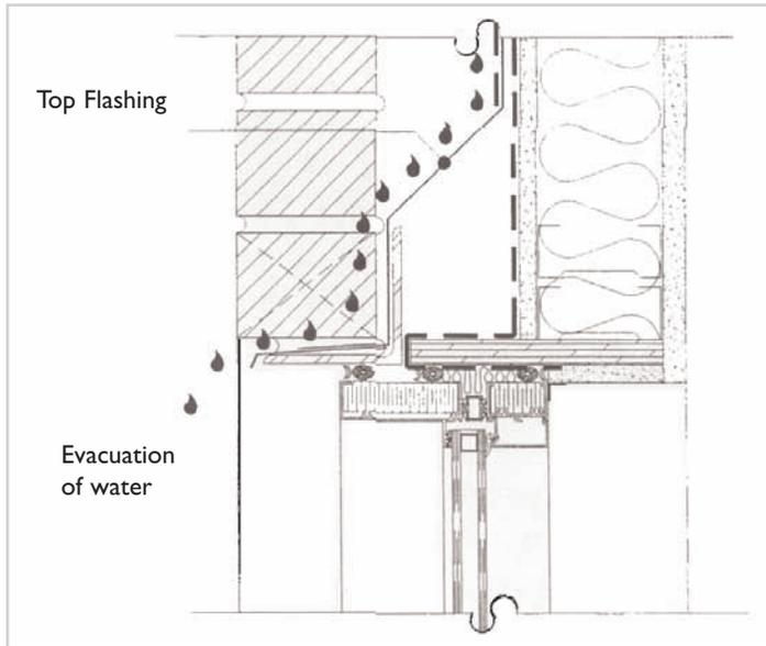
Figure 1 Top Flashing
