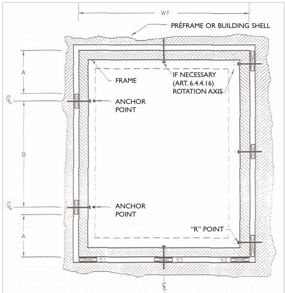
Figure 3 Shims for Casement Windows
